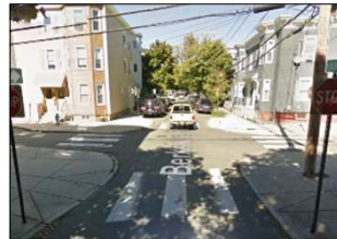
Motorist view of the curb extension at Berkshire and Plymouth Streets
