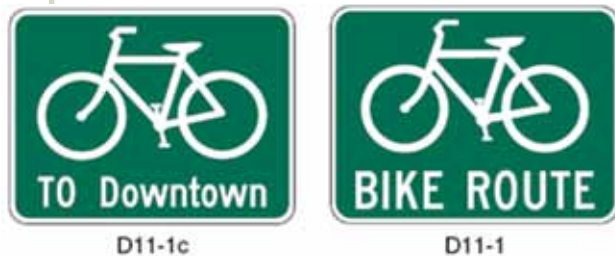
Figure 4-25. D11 Series Bicycle Route Signs
