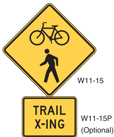
Figure 5-24. Advance Warning Assembly Example
