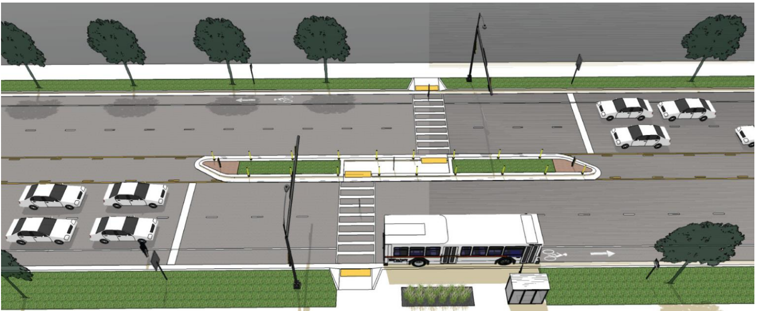
Figure 19. Graphic. Rendering of urban five-lane arterial with midblock crosswalk and transit stop similar to the example scenario. Source: The Greenway Collaborative, Inc.
