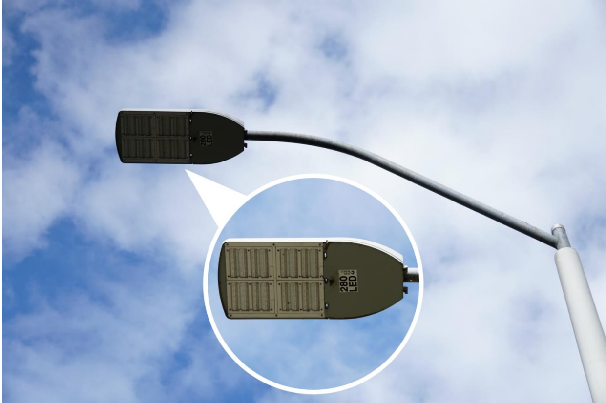
Figure 20. Graphic. Example LED cobrahead roadway luminaire. Source: FHWA.
