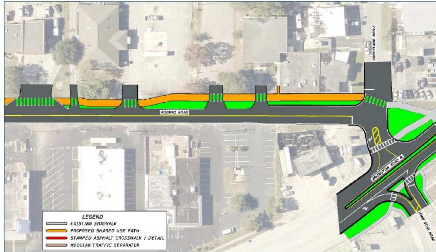
Figure 8 - Detail of Roll Plot (Segment 1)
