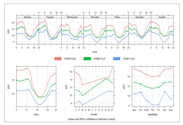
Figure 91. H<sub>2</sub>S hourly, daily, weekly, and monthly cycles at SYM3 – eNose 3, SYM2 – eNose 4, SYM1 – eNose 5.
