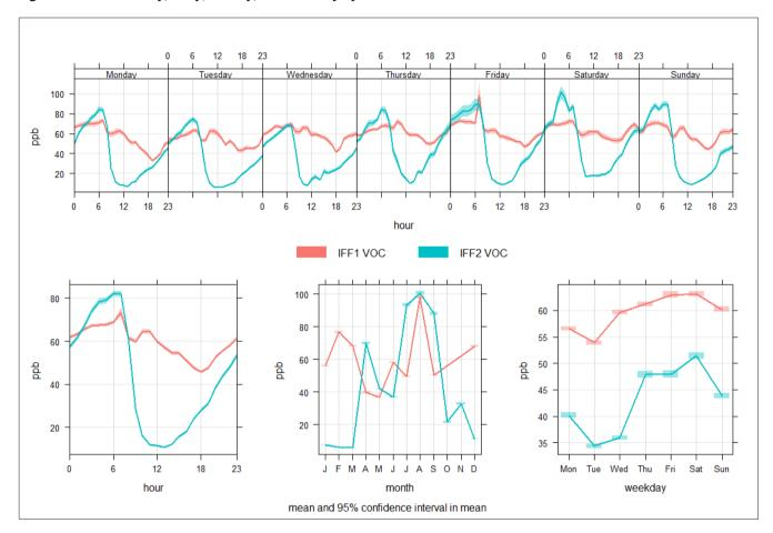
Figure 111. VOC hourly, daily, weekly, and monthly cycles at IFF - eNose 6 and IFF - eNose 7.
