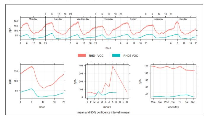
Figure 123. VOC hourly, daily, weekly, and monthly cycles at RHD1 - eNose 8 and RHD2 - eNose 9.
