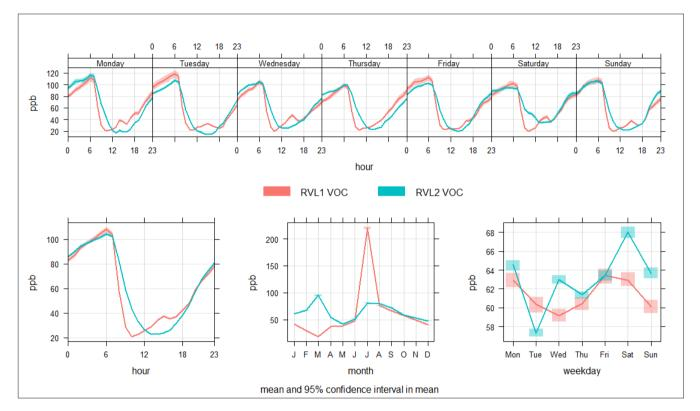
Figure 135. VOC hourly, daily, weekly, and monthly cycles at RVL1 – eNose 10 and RVL2 – eNose 11.
