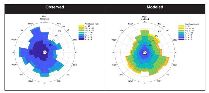
Figure 140. Observed and modeled wind roses at Met 1.
