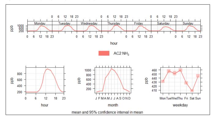
Figure 71. NH<sub>3</sub> hourly, daily, weekly, and monthly cycles at AC2 – eNose 2.
