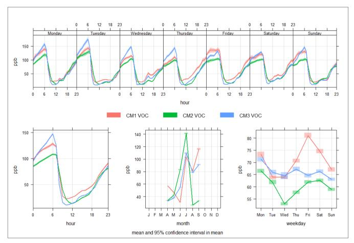
Figure 87. VOC hourly, daily, weekly, and monthly cycles at CM1 - eNose 3, CM2 - eNose 4, CM3 - eNose 5.
