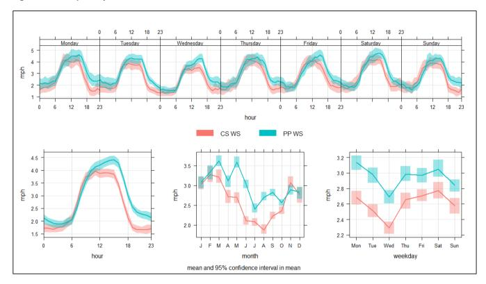
Figure 7. Wind speed cycles for CS and PP stations. Historical Data.
