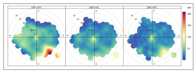
Figure 88. VOC pollution roses at CM1 – eNose 3, CM2 – eNose 4, CM3 – eNose 5.
