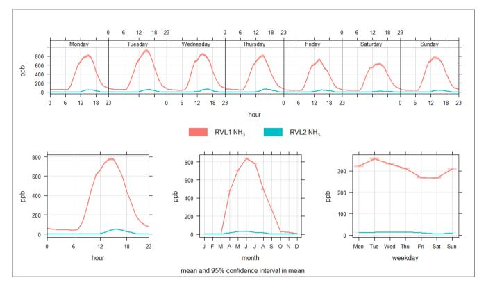
Figure 131. NH<sub>3</sub> hourly, daily, weekly, and monthly cycles at RVL1 – eNose 10 and RVL2 – eNose 11.
