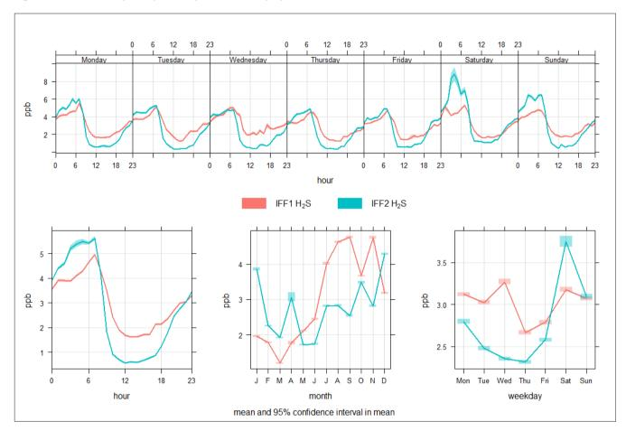
Figure 103. H<sub>2</sub>S hourly, daily, weekly, and monthly cycles at IFF – eNose 6 and IFF – eNose 7.
