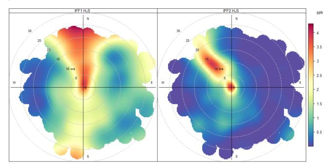
Figure 104. H<sub>2</sub>S pollution roses at IFF – eNose 6 and IFF – eNose 7.
