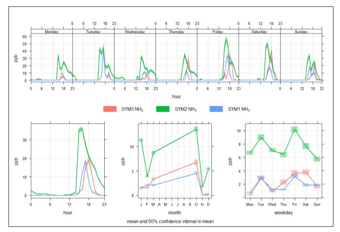
Figure 95. NH<sub>3</sub> hourly, daily, weekly, and monthly cycles at SYM3 – eNose 3, SYM2 – eNose 4, SYM1 – eNose 5.
