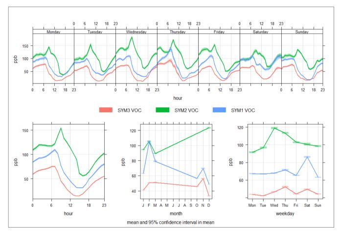
Figure 99. VOC hourly, daily, weekly, and monthly cycles at SYM3 – eNose 3, SYM2 – eNose 4, SYM1 – eNose 5.
