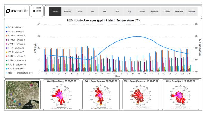
Figure 46. Example of page 6 of the monthly report showing H2S and temperature hourly averages and wind roses.
