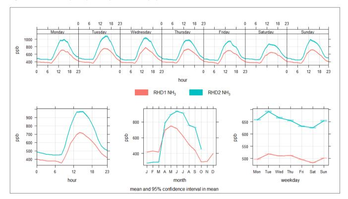
Figure 119. NH<sub>3</sub> hourly, daily, weekly, and monthly cycles at RHD1 – eNose 8 and RHD2 – eNose 9.
