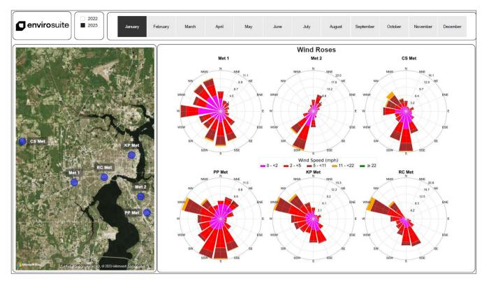
Figure 48. Example of page 8 of the monthly report showing wind roses for each weather station.
