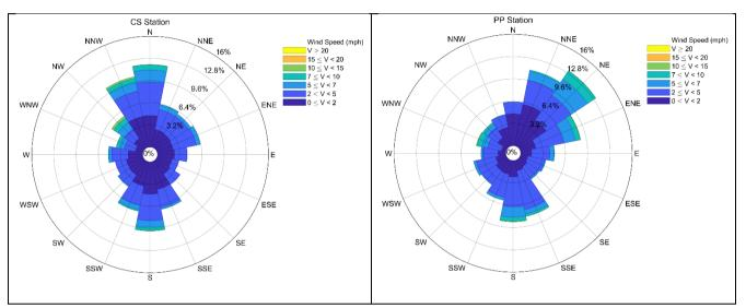
Figure 5. Wind speed and wind direction wind roses for CS and PP stations, full period. Historical Data.
