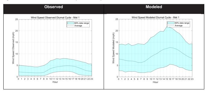
Figure 138. Observed and modeled wind speed diurnal cycles at Met 1.
